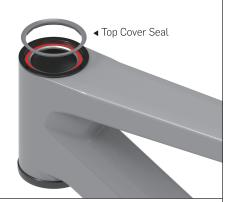
Assemble the proper housing seals (grommets) or port plug as needed onto the headset top cover.
