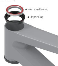
Apply a thin layer of lubricant to the inner edge of the upper cup, then assemble the seal. The seal lip should be facing up.
