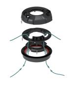
Complete the installation of the M-BOX headset – including the compression ring as shown on the right.
